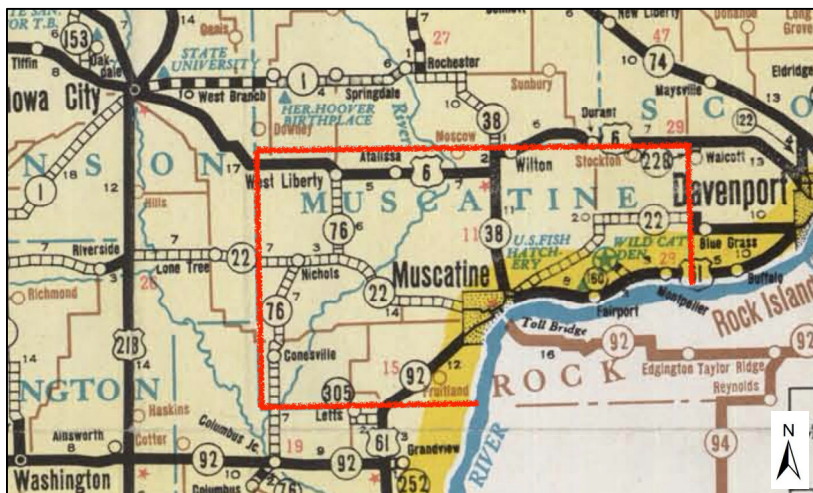
Figure 42. State of Iowa Map, 1940, showing the progress Muscatine County had made in paving (heavy black lines) the state and federal highways within its borders (red lines). Only State Highways 22 and 76 remained gravel-surfaced (segmented lines). Source: Iowa DOT Historic Maps
