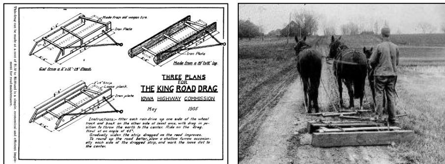
Figure 22. Left - Diagram of the King Road Drag with instructions by the Iowa State Highway Commission, 1905; Right - the King Road Drag in use. Sources: Left - Iowa Highway Commission 1905; Right – Minnesota Historical Society/Stilgoe-National Humanities Center
